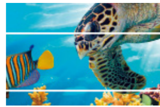
Gap/White streaks (Excessive feeding amount)
